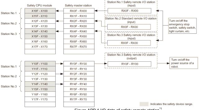
Figure APP.1 I/O data of safety remote station<sup>\*1</sup>
