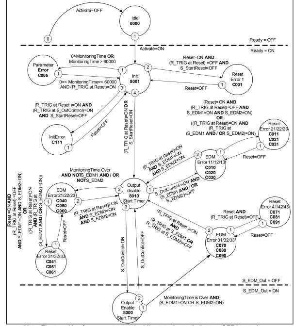
Note: The transition from any state to the Idle state due to Activate = OFF is not shown. However these transitions have the highest priority (0). Figure 4.7 State Diagram for S+EDM
