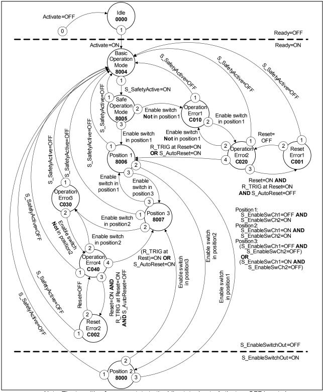
Note: The transition from any state to the Idle state due to Activate = OFF is not shown. However these transitions have the highest priority (0). Figure 4.10 State Diagram for S+ENBLSW
