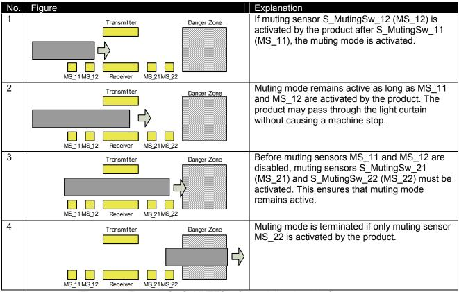
Figure 4.42 Example for S+MUTES in forward direction with four sensors
