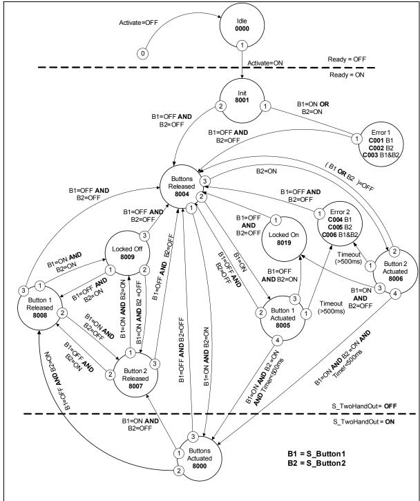
Note: The transition from any state to the Idle state due to Activate = OFF is not shown. However these transitions have the highest priority (0). Figure 4.4 State Diagram for S+2HAND3
