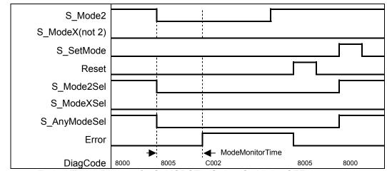
Figure 4.32 Typical Timing Diagram for S+MODSEL (S\_AutoSetMode=OFF) Error condition 2 at Mode inputs (All S\_ModeX=OFF after ModeMonitorTime)
