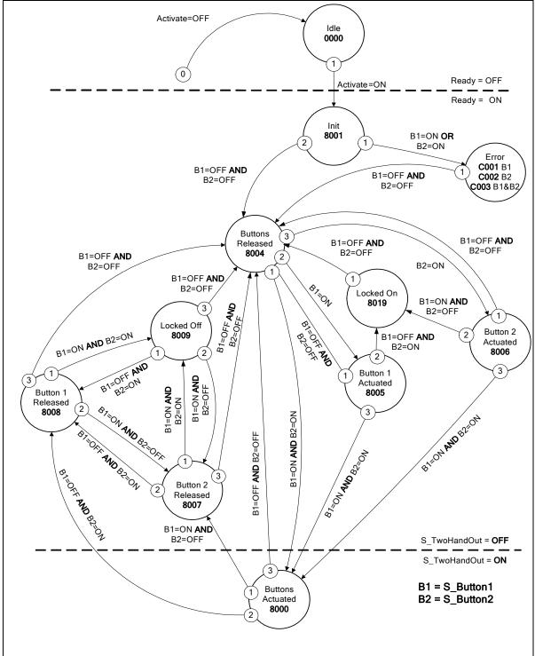
Note: The transition from any state to the Idle state due to Activate = OFF is not shown. However these transitions have the highest priority (0). Figure 4.1 State Diagram for S+2HAND2
