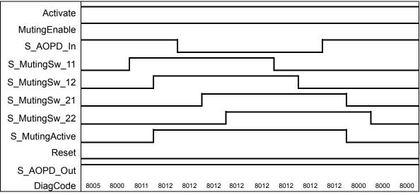
Figure 4.44 Tyical Timing Diagram for S+MUTES (forward direction)
