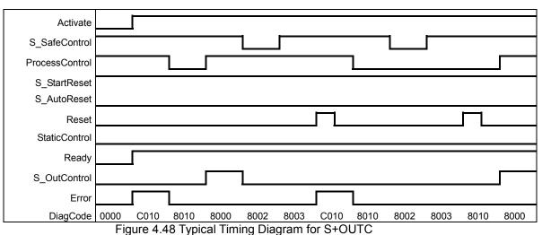
Igure 4.48 Typical Timing Diagram for S+OUT S\_StartReset=ON, S\_AutoReset = OFF
