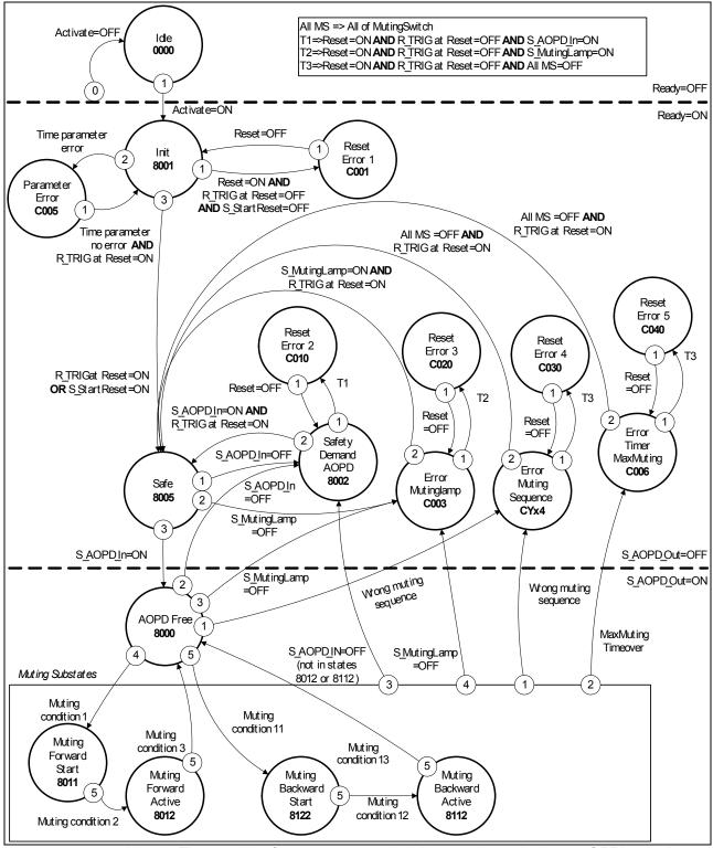
Note 1: The transition from any state to the Idle state due to Activate = OFF is not shown. However these transitions have the highest priority (0).
