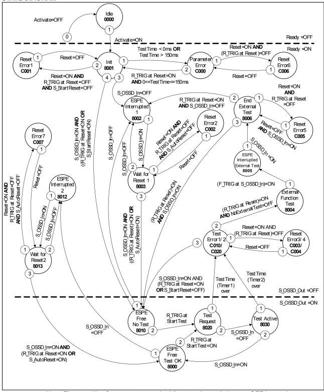
Note: The transition from any state to the Idle state due to Activate = OFF is not shown. However these transitions have the highest priority (0). Figure 4.50 State Diagram for S+TSSEN
