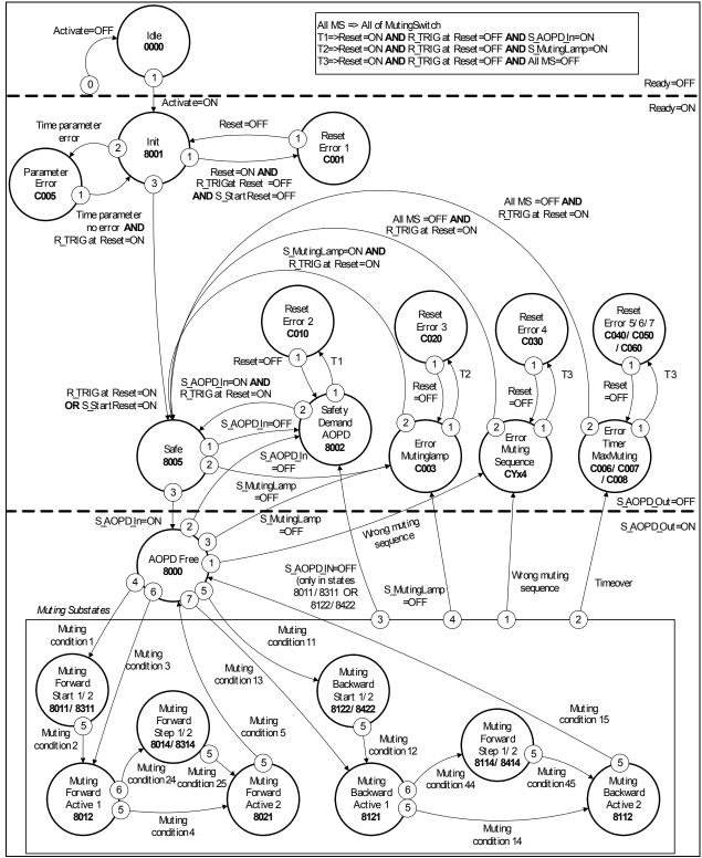
Note1: The transition from any state to the Idle state due to Activate = OFF is not shown. However these transitions have the highest priority (0).
