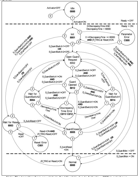
Note: The transition from any state to the Idle state due to Activate = OFF is not shown. However these transitions have the highest priority (0). Figure 4.26 State Diagram for S+GMON
