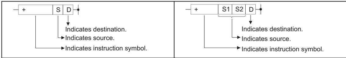
Fig. 2.1 Shows Symbol Diagram on the Ladder
