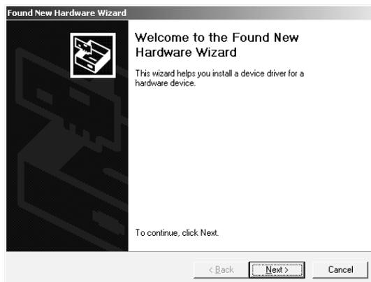
1) The screen shown on the left appears when you connect the personal computer and QCPU (Q mode) by the USB cable.
