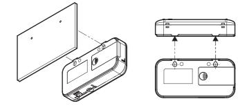
There are two hook holes below the convex section of the upper unit. Use M3 screws to hook the screw head on the screw hook holes. Set an interval of 2.5 mm or more between the bottom of the screw head and the wall surface.
