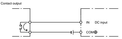
When using the configuration shown below, the sensor and Input Unit should receive their power from the same supply.
