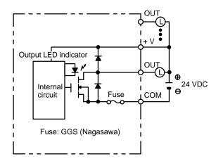
Note No blown fuse detector circuit is provided.
