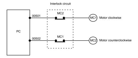
This circuit prevents outputs MC1 and MC2 from ever both being ON at the same time. Even if the PC is programmed improperly or malfunctions, the motor is protected.
