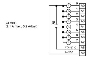
Note Be sure to supply power to A9; otherwise current will leak through the load while the output is OFF.
