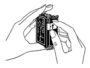
3. Pull the printed circuit board out of the EPROM Pack.
