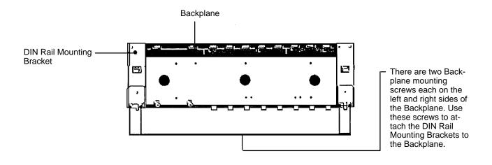
2. Mount the Backplane to the DIN Rail so that the claws on the Mounting Brackets fit into the upper portion of the DIN Rail as shown below.
