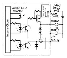
**Note** When short-circuit/overload protection is activated, all 16 outputs will be switched OFF and the ALARM output becomes active (low level). The problem can be detected externally by connecting a DC Input Unit to the ALARM output or by connecting an alarm output indicator. It's not possible to connect both the Input Unit and the indicator at the same time.
