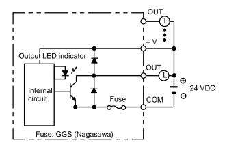
Note No blown fuse detector circuit is provided.
