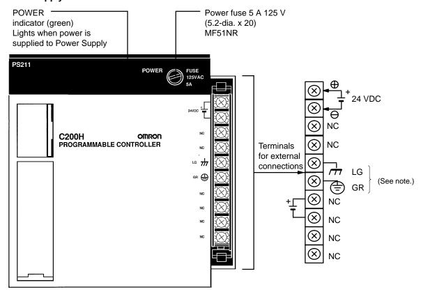
Note The LG and GR terminals are connected internally.
