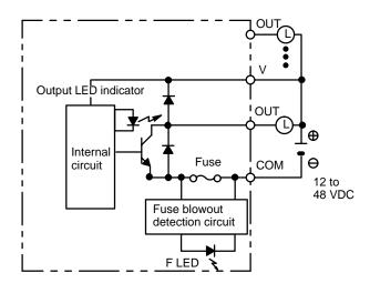
Note When the fuse blows F LED lights and bit 08 turns ON. Bits 08 through 15 cannot be used as work bits.
