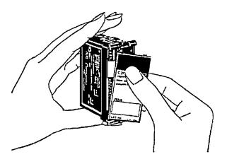
2. Unlock the holding bracket and slide it upward to remove it as shown below
