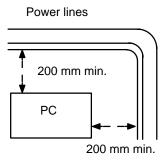
Whenever possible, use wiring conduit to hold the I/O wiring. Standard wiring conduit should be used, and it should be long enough to completely contain the I/O wiring and keep it separated from other cables.
