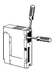
6. Pull out the printed circuit board. The Relays are placed on the PC boards of individual Units as shown in the figures below.
