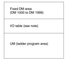
**Note** I/O tables are also saved in the Memory Unit at the time of creation. Therefore, if the Memory Unit is set to write-protect, it will be impossible to create an I/O table.
