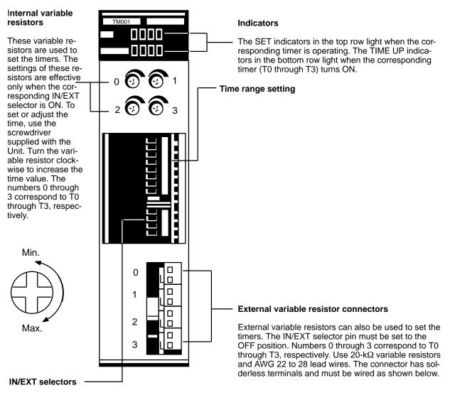
When the internal variable resistor is used, set the corresponding pin to ON; when an external variable resistor is used, set the corresponding pin to OFF. Pin numbers 4 through 1 correspond to T0 through T3, respectively.
