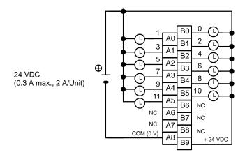
Note Be sure to supply power to B9; otherwise current will leak through the load while the output is OFF.
