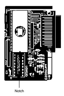
5. Reassemble the EPROM Pack in the reverse order of disassembly. During reassembly, ensure that the circuit board is inserted along the guides on the top and bottom of the Pack housing and that the projections on the housing fit into the holes in the holding bracket. Be sure to lock the holding bracket into the right side of the housing. When reassembled, the Pack should appear as shown below.
