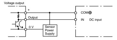
The circuit below should **NOT** be used for I/O devices having a voltage output.
