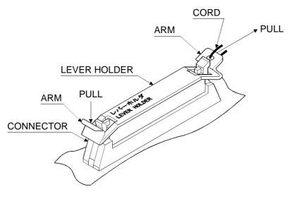
When removing, if pulled out with force using only the cord, the lever holder will come out with force and may cause injuries.
