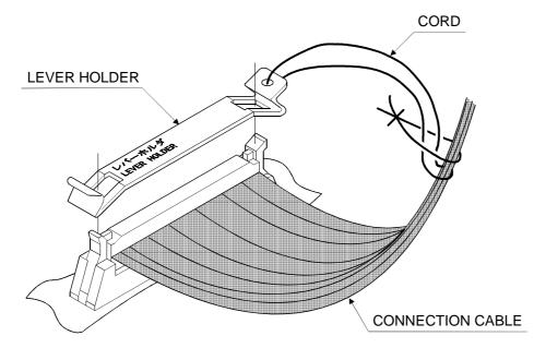
(2) Place the both holes of the Lever Holder on top of connector levers and position the Lever Holder on connector.
