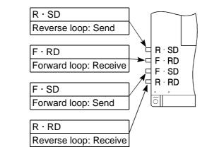
• Connect the coaxial cable connector and cables as shown below.
