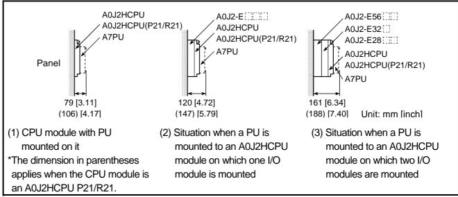
Fig. 3.1 Dimensions for Module-to-Module Mounting
