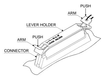
(4) Check to ensure that the Lever Holder is firmly attached the connector and locked connector levers.
