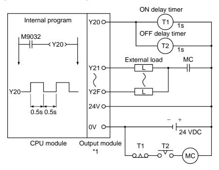
\*1 As "Y20" repeatedly switches ON and OFF at 0.5 second intervals, a non-contact output module ("transistor" in the above example) should be used.
