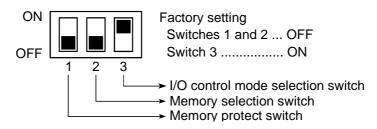
Setting the memory protect switch The memory protect range is the first 20k bytes of the 32k byte user memory area.
