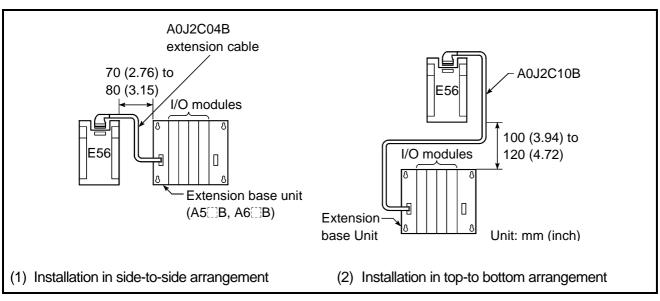
Fig3.4 Installation of Extension Base Unit
