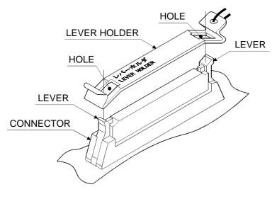
(3) Using fingers, push arms of the Lever Holder to lower top of connector levers and lock connector levers.
