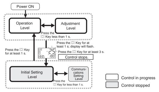
This level is displayed immediately after the power is turned ON. To move to other levels, press the O key or the O and M keys.
