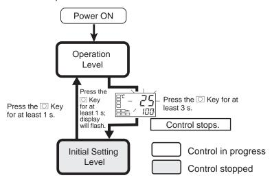
To move from the operation level to the initial setting level, press the O key for at least 3 seconds with any parameter displayed except for the "auto/manual switch" parameter.
