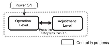
To move to the adjustment level from the operation level, press the  $\ensuremath{\bigcirc}$  key once.
