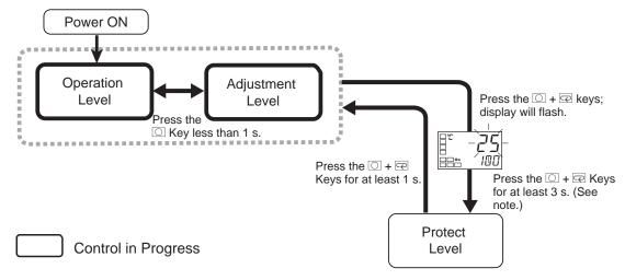
To move from the operation level to the protect level, press  $\bigcirc$  and M keys for three seconds (See note.) or more.
