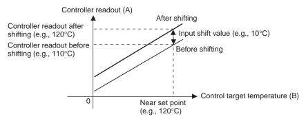
Figure 2 Illustration of 1-Point Shift
