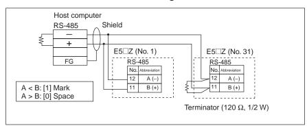
The RS-485 connection can be either one-to-one or one-to-N. A maximum of 32 Units (including the host computer) can be connected in one-to-N systems. The maximum total cable length is 500 m. Use AWG24 (cross-sectional area: 0.205 mm²) to AWG14 (cross-sectional area: 2.081 mm²) shielded twisted-pair cable.
