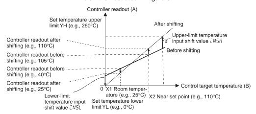
Figure 3 Illustration of 2-Point Shift
