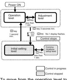
To move from the operation level to the initial setting level, press key for three seconds or more.
