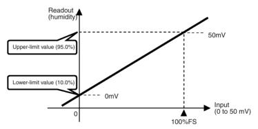
In this example, let's set the scaling upper- and lower-limits so that inputs 0 to 50 mV become 10.0% to 95.0%.
