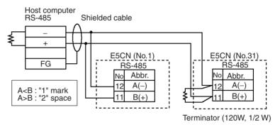
The RS-485 connection can be either one-to-one to one-to-N. Up to 32 units including the host computer can be connected in one-to-N systems.
