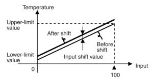
In this example, let's shift the input of the K sensor by "1°C" by 1-point input shift.
