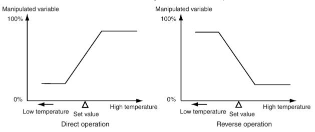
For example, when the process value (PV) (temperature) is lower than the set point (SP) (temperature) in a heating control system, the manipulated variable increases by the difference between the PV and SP values.
