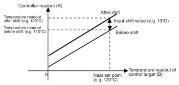
Figure 2 1-point Temperature Input Shift
