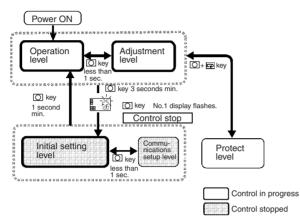
To move to the adjustment level from the operation level, press the key for less than one second.
