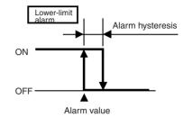
• Alarm hysteresis is set independently for each alarm in the "alarm hysteresis 1" and "alarm hysteresis 2" parameters (advanced function setting level). Default is "0.2".
