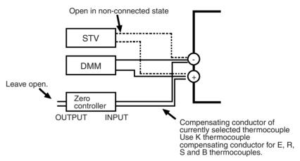
Disconnect the STV to enable the thermocouple of the cold junction compensator. When doing this, be sure to disconnect the wiring on the STV side
