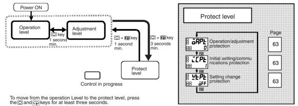
The settings of protected parameters are not displayed and so cannot be modified.
