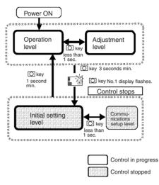
This level is automatically displayed immediately after the E5CN is turned ON. To move to other levels, press
