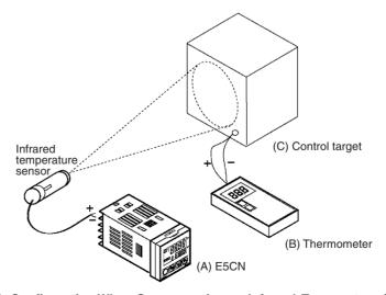
Figure 1 Configuration When Compensating an Infrared Temperature Sensor
