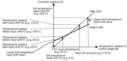
Figure 3 2-point Temperature Input Shift
