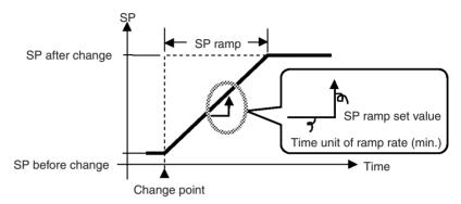
The change rate during SP ramp is specified by the "SP ramp set value" parameter. The "SP ramp set value" default is "OFF", and the SP ramp function is disabled.
