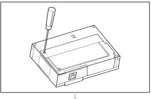
1) Loosen the mounting screws (2 pcs.) that fix the slot cover on the back of the A9GT-J71E71-T.
