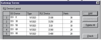
When 100 points of devices are accessed, access to the PLC must be made five times.
