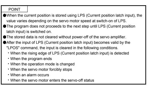
The current position at switch-on of LPS (Current position latch input) is stored. The stored position data can be read with the communication function.
