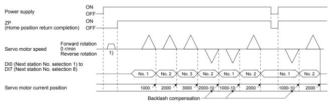
Backlash is compensated to the direction set with [Pr. PT38] regardless of a JOG operation (1)) or disturbance after power-on.
