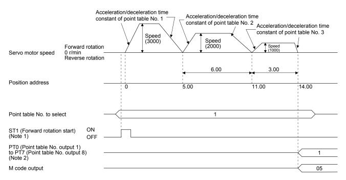
Note 1. Switching on ST2 (Reverse rotation start) starts positioning in the reverse rotation direction.
