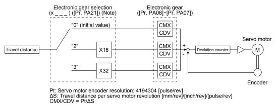
Note. For MR-J4-03A6-RJ servo amplifiers, "2 \_ \_ " or "3 \_ \_ " cannot be set to [Pr. PA21].
