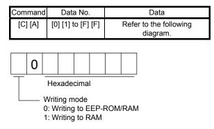
When the dwell is changed frequently using communication, set "1" to the mode to change only the RAM data in the servo amplifier.
