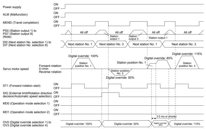
Note. For MR-J4-03A6-RJ servo amplifiers, up to six points of DO are available; therefore, PS0 to PS7 cannot be outputted simultaneously.
