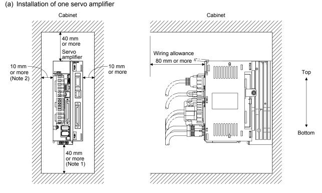
Note 1. For the 11 kW to 22 kW servo amplifiers, the clearance between the bottom and the ground will be 120 mm or more. 2. For the MR-J4-500A-RJ, the clearance between the left side and wall will be 25 mm or more. (b) Installation of two or more servo amplifiers
