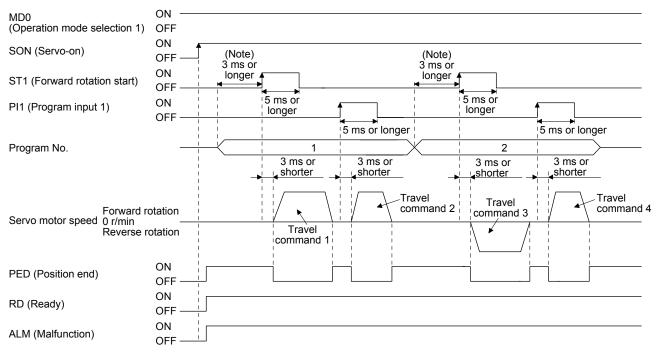
Note. The detection of external input signals is delayed by the set time in the input filter setting of [Pr. PD29]. Considering the output signal sequence from the controller and signal variations due to hardware, configure a sequence that changes the program selection earlier.
