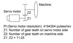
7.3.2 Electronic gear setting in the indexer method
