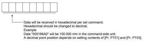
(b) Rising latch data or falling latch data (data part + additional information) Reads MSD (Mark detection) rising latch data or MSD (Mark detection) falling latch data.
