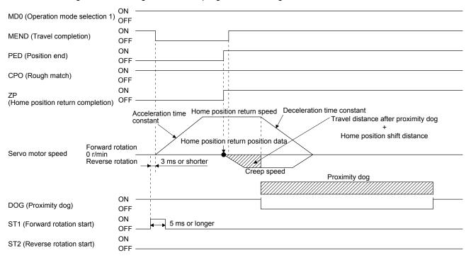
The setting value of [Pr. PT08 Home position return position data] is used as the position address at the home position return completion.
