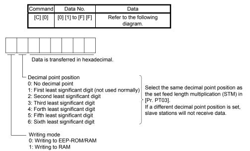
When the position data is changed frequently using communication, set "1" to the mode to change only the RAM data in the servo amplifier.
