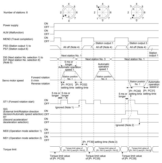
Note 1. When the rest of command travel distance is other than "0", ST1 (Forward rotation start) will not be accepted. Refer to section 6.4.5 (1).
