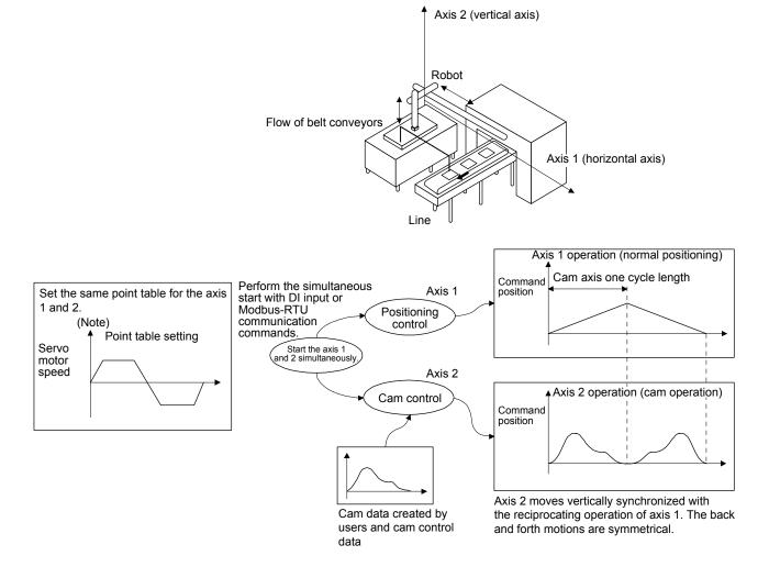
Note. Input the same positioning commands (point table data) to the driven shaft (axis 2) as those for the main shaft (axis 1).
