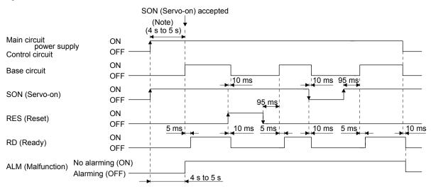
Note. The time will be longer during the magnetic pole detection of a linear servo motor and direct drive motor.
