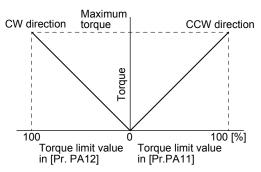
A relation between the applied voltage of OTLA (Analog torque limit) and the torque limit value of the servo motor is as follows. Torque limit values will vary about 5% relative to the voltage depending on products. At the voltage of less than 0.05 V, torque may vary as it may not be limited sufficiently. Therefore, use this function at the voltage of 0.05 V or more.
