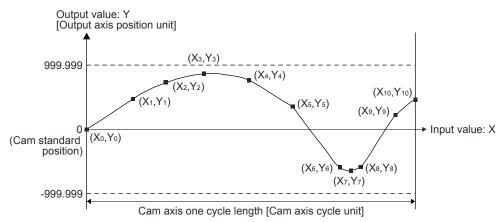
If "input value = 0" and "input value = cam axis one cycle length" are not set in the coordinate data, a control is executed by the line connecting the closest two points.
