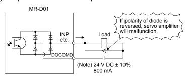
Note. If the voltage drop (maximum of 2.6 V) interferes with the relay operation, apply a high voltage (maximum of 26.4 V) from an external source.
