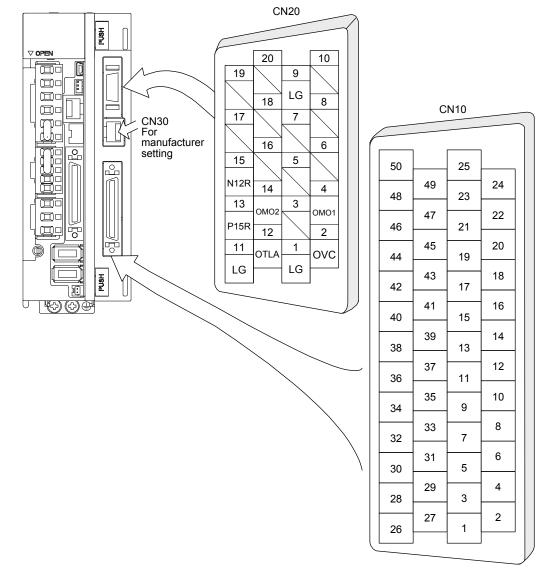
For the pin assignment, refer to (3) of this section.
