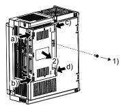
1) Find the guide hole on the side of the servo amplifier. To the guide hole, insert the MR-D01's guide pins.
