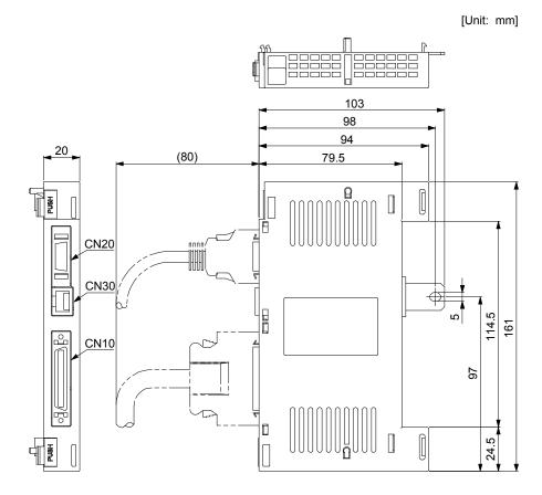
11.8.2 When an MR-D01 extension IO unit is connected to a servo amplifier
