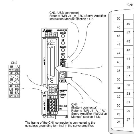
The device assignment of the CN1 connector pins changes depending on the control mode. For the pins which are given parameters in the related parameter column, their devices can be changed using those parameters.
