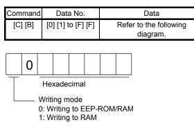
When the sub function is changed frequently using communication, set "1" to the mode to change only the RAM data in the servo amplifier.
