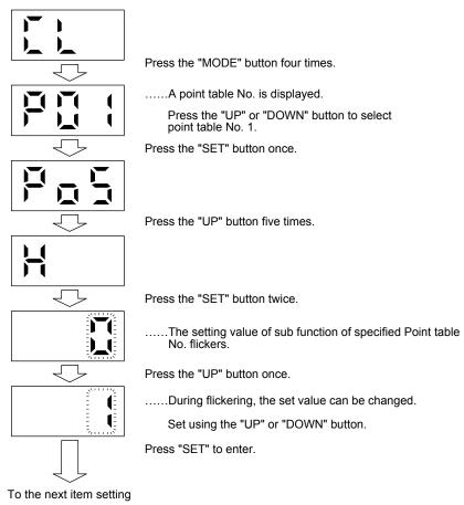
Press the "UP" or "DOWN" button to switch to other item of the same point table No. Press the "MODE" button to switch to the next point table No. (b) Setting of 4 to 6 digits
