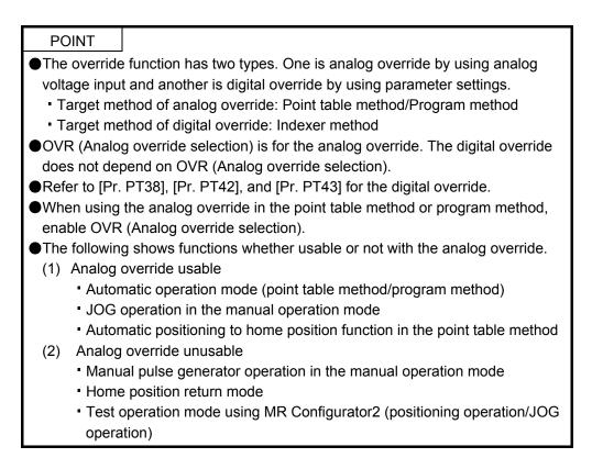
You can change the servo motor speed by using VC (Analog override). The following table shows signals and parameters related to the analog override.
