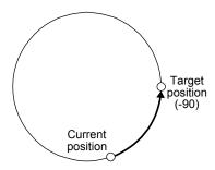
If the position data of 270.000 degrees is specified when the current position is at 90, the distances in the CCW and CW are the same. In such a case, the servo motor rotates in the CCW direction.
