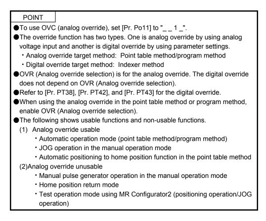
You can change the servo motor speed by using OVC (Analog override). The following table shows signals and parameters related to the analog override.
