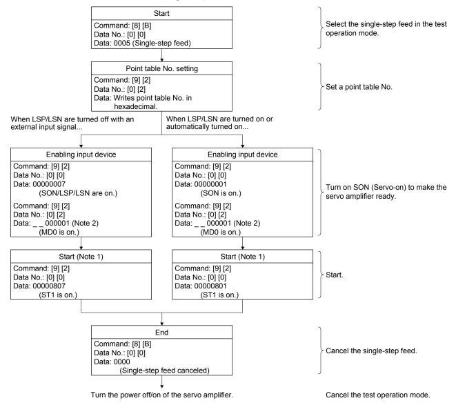
Note 1. After checking ZP (Home position return completion), start it. See the 4 bit of the read data with the command [1] [2] and data No. [8] [2].
