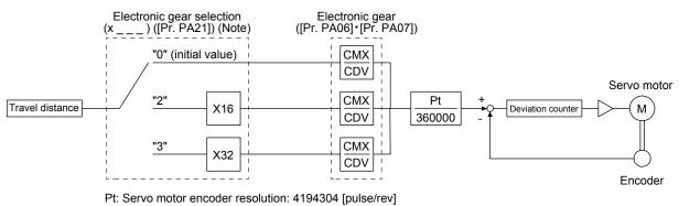
Note. For MR-J4-03A6-RJ servo amplifiers, "2 \_ \_ " or "3 \_ \_ " cannot be set to [Pr. PA21].
