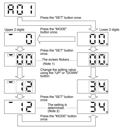
Note 1. Pressing the "SET" button in upper, middle, or lower 2-digit display makes the display flicker.
