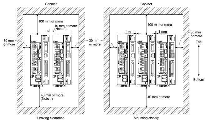
Note 1. For the 11 kW to 22 kW servo amplifiers, the clearance between the bottom and the ground will be 120 mm or more.
