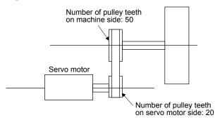
(2) Number of pulley teeth on machine side: 50, number of pulley teeth on servo motor side: 20, with geared servo motor of 1/9
