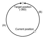
b) When using the shortest rotation specification ([Pr. PT03] = \_ 1 \_ \_)
