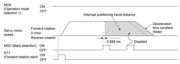
Note. Deceleration time constant of the point table at the time of start is applied for the point table method, and deceleration time constant set by the program in execution is applied for the program method.
