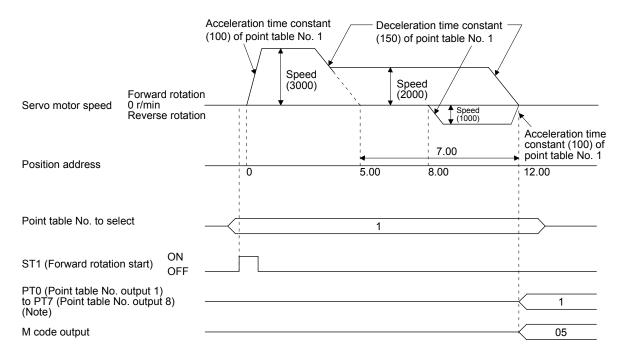
2) Incremental value command method ([Pr. PT01] = \_ \_ 1)
