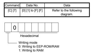
When the acceleration time constant is changed frequently using communication, set "1" to the mode to change only the RAM data in the servo amplifier.
