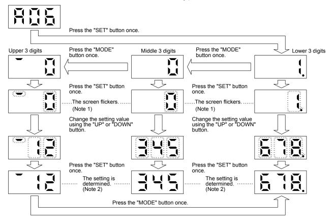
Note 1. Pressing the "SET" button in upper, middle, or lower 3-digit display makes the display flicker.
