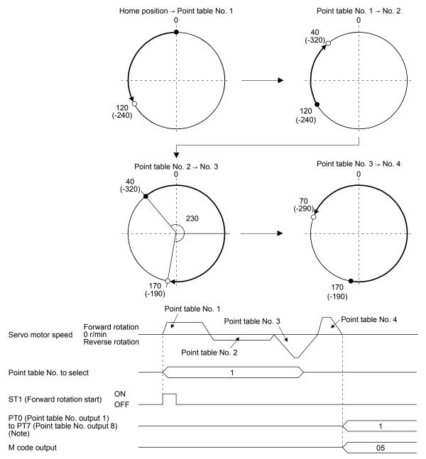
2) Incremental value command method ([Pr. PT01] = \_ \_ 1)
