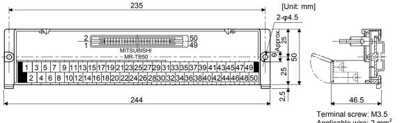
Applicable wire: 2 mm<sup>2</sup> Crimp terminal width: 7.2 mm or less
