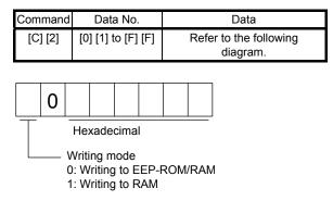
When the M code is changed frequently using communication, set "1" to the mode to change only the RAM data in the servo amplifier.
