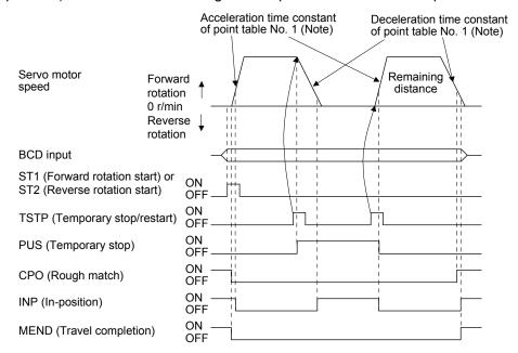
Note. When SPD1 (Speed selection 1) to SPD4 (Speed selection 4) are used, the acceleration/deceleration time constants of the point table selected at the start are used.
