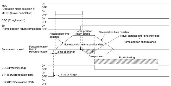
The setting value of [Pr. PT08 Home position return position data] is used as the position address at the home position return completion.
