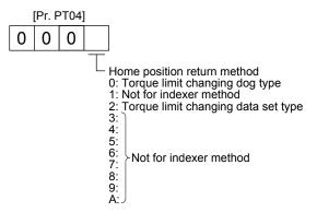
(b) Select the starting direction for the home position return with [Pr. PT04 Home position return type]. Setting "0" starts the home position return in the address increasing direction from the current position. Setting "1" starts the home position return in the address decreasing direction from the current position.
