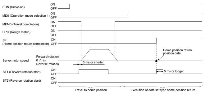
The setting value of [Pr. PT08 Home position return position data] is used as the position address at the home position return completion.
