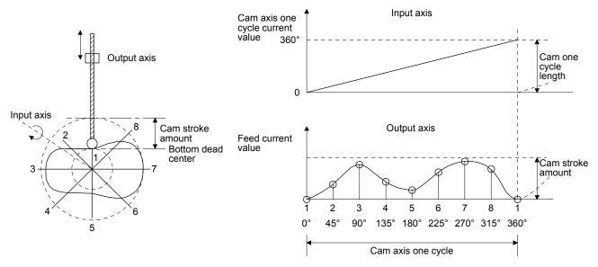
By setting cam data and cam control data, the simple cam function enables synchronous control with an input axis (external pulse command input, point table command, or program positioning command) with a start of positioning.
