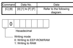
When the deceleration time constant is changed frequently using communication, set "1" to the mode to change only the RAM data in the servo amplifier.
