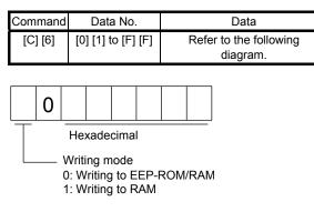
When the speed data is changed frequently using communication, set "1" to the mode to change only the RAM data in the servo amplifier.
