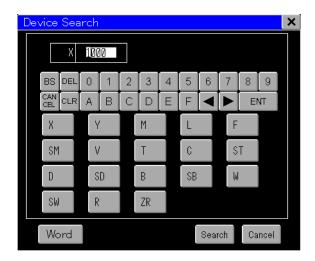
4 The ladder programs will be displayed starting with the device for which the alarm sounded.
