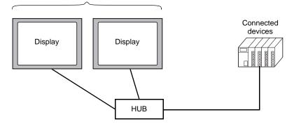
\* When the "Open Setting" function is used for the connected device instead of the "Auto Open UDP Port" function, up to 16 displays can be connected. However, when the "Auto Open UDP Port" function is used for the connected device, there is no limit on the number of connected displays.
