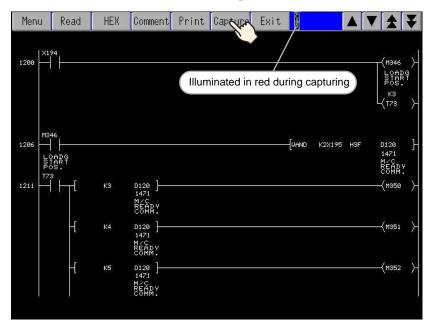
**2** The displayed screen is captured and saved on the CF Card. The file name is "CP\*\*\*\*.jpg" and \*\*\*\*\* is an automatically assigned number from 0 to 65535.
