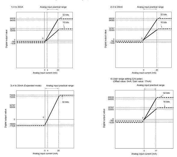
Fig. 3.2 Current input characteristic of Q64AD-GH
