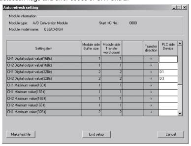
(c) Writing the intelligent function module parameters (see Section 5.3.3) Write the intelligent function module parameters to the CPU module. This operation is performed using the parameter setting module selection screen.
