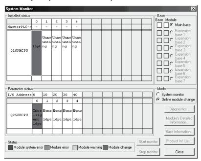
(d) Referring to (1), set the used channel to conversion enable, and monitor the digital output values (buffer memory addresses 11 to 14, 54 to 62, Un\G11 to 14, Un\G54 to 62) to check whether proper conversion has been made or not.
