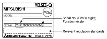
(b) To check the function version and product information using GX Developer Refer to Section 8.2.6 of this manual.
