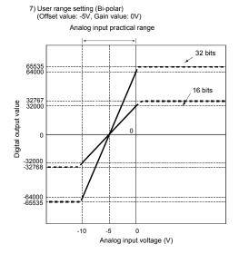
Fig. 3.1 Voltage input characteristic of Q64AD-GH (2/2)
