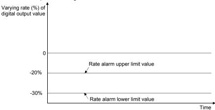
3) Example of setting the rate alarm upper limit value/lower limit value when it is desired to watch that the digital output value is at the varying rate within the specified range
