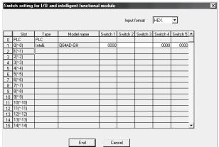
(b) Switch setting for intelligent function module screen
