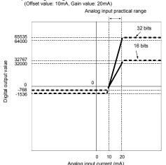
Fig. 3.3 Input characteristic of Q62AD-DGH
