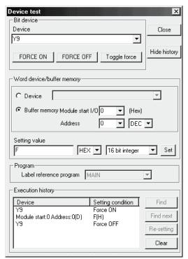
(The screen shows the setting example of the Q64AD-GH.)
