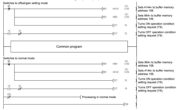
(c) When switching the mode by making intelligent function module switch setting
