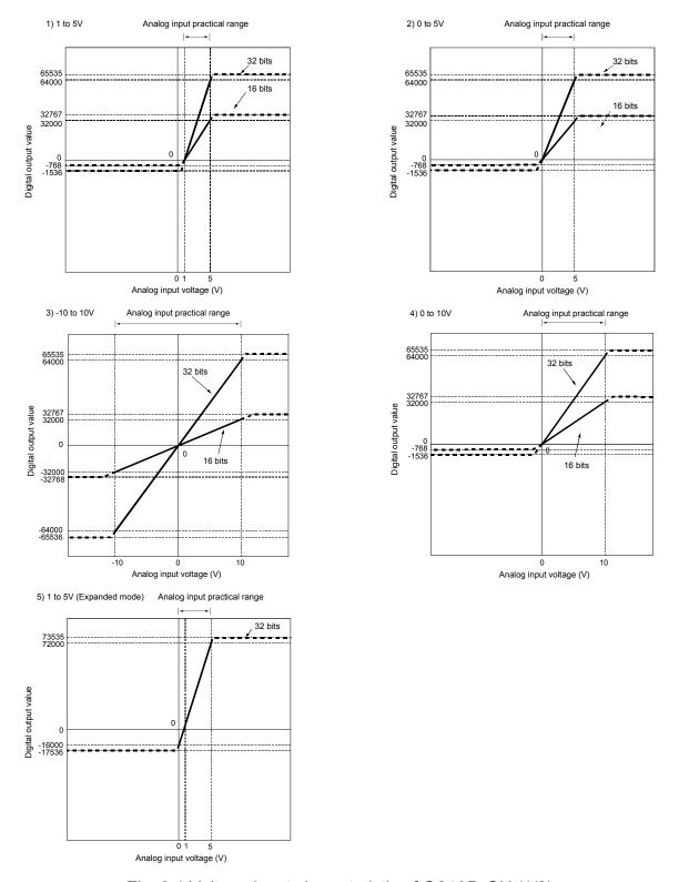
Fig. 3.1 Voltage input characteristic of Q64AD-GH (1/2)
