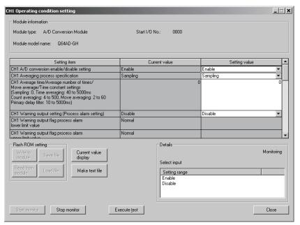
(b) After making sure that the indication in the Current value field of CH A/D conversion enable/disable setting is "Disable", change the Setting value field of Operating condition setting request to "Setting request", and click the [Execute test] button to stop conversion.
