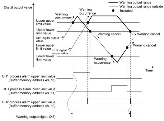
(c) When time or count averaging is specified, this function is executed at intervals of the preset averaging time or averaging count. When any other A/D conversion system (sampling processing, move averaging, primary delay filter) is specified, this function is executed at intervals of the sampling time.
