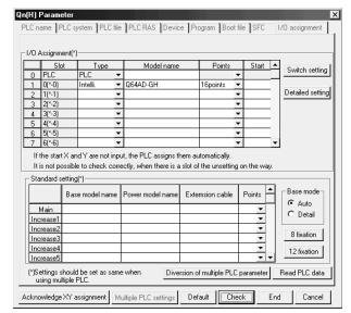
(a) I/O assignment setting screen Set the following for the slot in which the A/D converter module is mounted.
