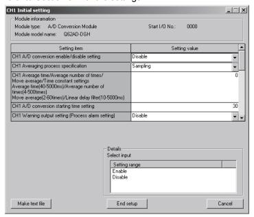
(b) Auto refresh setting (see Section 5.5) Set the digital output values, warning output flags, input signal error detection flags and error codes of CH1 and 2.
