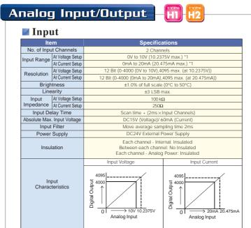
\*1 Switching the Voltage Input or Current Input can be set separately, in each channel.
