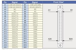
\* This front diagram shows the connector on the DIO unit side. When preparing the cable, note that the (a) and (b) characters indicate the number 1 pins.
