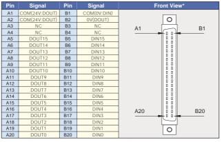
\* This front diagram shows the connector on the DIO unit side. When preparing the cable, note that the and characters indicate the number 1 pins.
