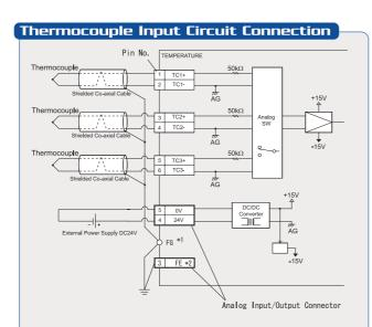
\*1 Connect to the FG terminal in the main unit, or connect directly to frame ground (FG). \*2 Ground this wire when noise or other problems occur during unit operation.
