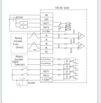
\*1 The FN-PC unit's live line is not isolated. If it is connected to a non-isolated servo driver, be sure to connect the signal ground (5G) to prevent over-current damage.
