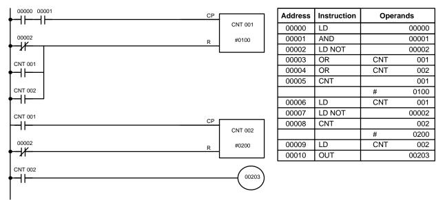
CNT can be used in sequence as many times as required to produce counters capable of counting any desired values.
