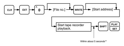
\*\*These times take the cassette leader tape into consideration according to the following: a) When recording to tape, the leader tape needs to be allowed to pass before the data transmission to the tape player starts.
