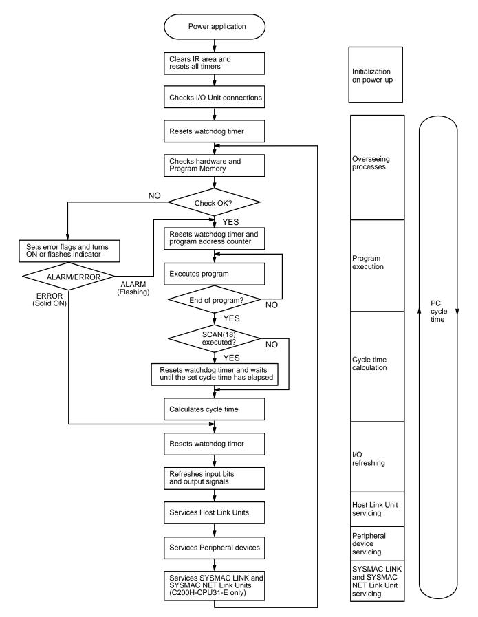
The first three operations immediately after power application are performed only once each time the PC is turned on. The rest of the operations are performed in cyclic fashion, with each scan forming one cycle. The cycle time is the time that is required for the CPU to complete one of these cycles. This cycle includes basically seven types of operation.
