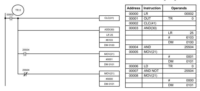
Although two ADD(30) can be used together to perform eight-digit BCD addition, ADDL(54) is designed specifically for this purpose.
