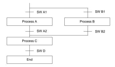
The program for this process, shown below, starts with two SNXT(09) instructions that start processes A and B. Because of the way 00001 (SW A1) and 00002 (SB B1) are programmed, only one of these will be executed to start either process A or process B. Both of the steps for these processes end with a SNXT(09) that starts the step for process C.
