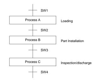
The program for this process, shown below, utilizes the most basic type of step programming: each step is completed by a unique SNXT(09) that starts the next
