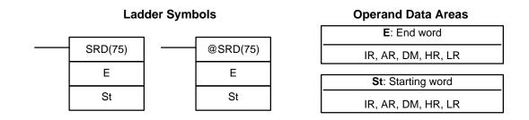
St and E must be in the same data area, and E must be less than or equal to St.
