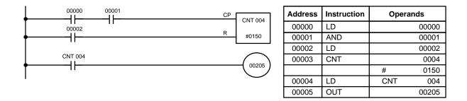
Here, 00000 can be used to control when CNT is operative and 00001 can be used as the bit whose OFF to ON changes are being counted.
