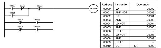
The following diagram requires five blocks, which here are coded in order before using OR LOAD and AND LOAD to combine them starting from the last two blocks and working backward. The OR LOAD at program address 00008 combines blocks blocks d and e, the following AND LOAD combines the resulting execution condition with that of block c, etc.
