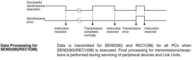
Programming Example: Multiple SEND(90)/RECV(98) To ensure successful SEND(90)/RECV(98) operations, your program must use the SEND(90)/RECV(98) Enable Flags and SEND(90)/RECV(98) Error Flags to confirm that execution is possible. The following program shows one example of how to do this for a SYSMAC NET Link System.
