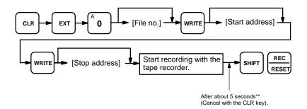
\*\*These times take the cassette leader tape into consideration according to the following: a) When recording to tape, the leader tape needs to be allowed to pass before the data transmission to the tape player starts. b) When restoring from tape or comparing data, the Programming Console needs to be ready to receive data before the data is transfered from the tape.
