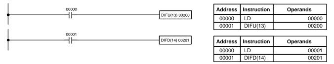
Here, IR 00200 will be turned ON for one cycle after IR 00000 goes ON. The next time DIFU(13) 00200 is executed, IR 00200 will be turned OFF, regardless of the status of IR 00000. With the DIFFERENTIATE DOWN instruction, IR 00201 will be turned ON for one cycle after IR 00001 goes OFF (IR 00201 will be kept OFF until then), and will be turned OFF the next time DIFD(14) 00201 is executed.
