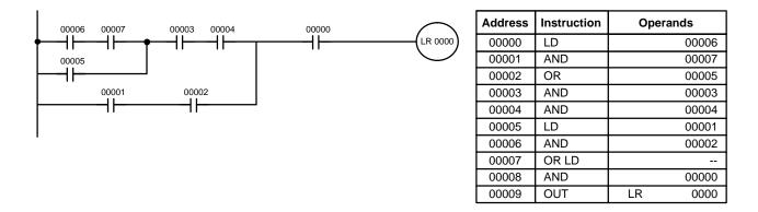
The next and final example may at first appear very complicated but can be coded using only two logic block instructions. The diagram appears as follows:
