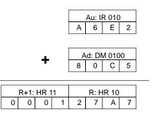
The following example performs eight-digit addition by using ADB(50) twice. ADB(50) is also used to place the carry into DM 0302 (one word greater than the rest of the answer). The complete answer thus ends up in DM 0300 through DM 0302.
