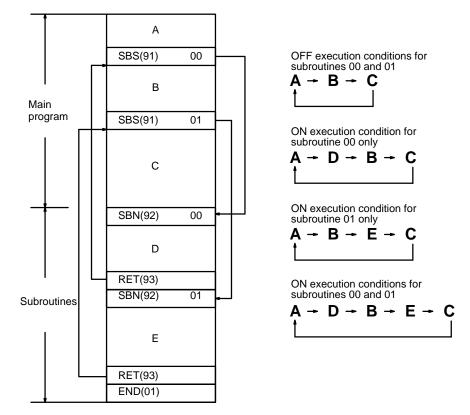
The following diagram illustrates program execution flow for various execution conditions for two SBS(91).
