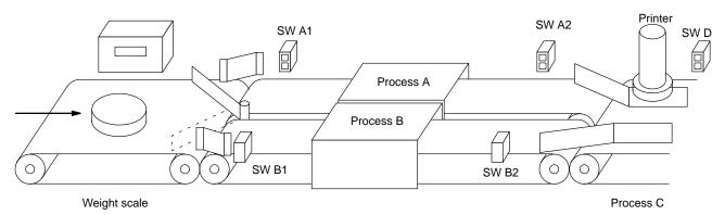
The following diagram demonstrates the flow of processing and the switches that are used for execution control. Here, either process A or process B is used depending on the status of SW A1 and SW B1.
