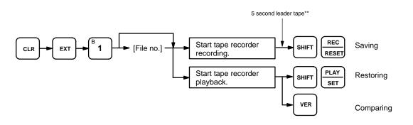
\*\*These times take the cassette leader tape into consideration according to the following: a) When recording to tape, the leader tape needs to be allowed to pass before the data transmission to the tape player starts.
