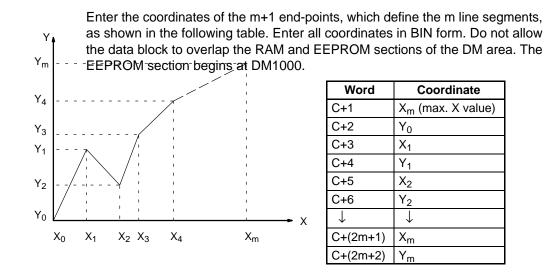
The following example demonstrates the construction of a linear approximation with 12 line segments. The block of data is continuous, as it must be, from DM 0000 to DM 0026 (C to C +  $(2 \times 12 + 2)$ ). The input data is taken from IR 010, and the result is output to IR 011.
