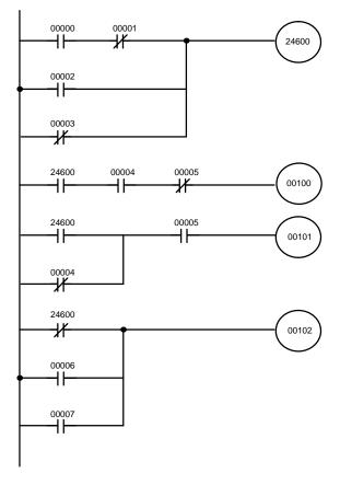
output conditions for IR 00100, IR 00101, and IR 00102, i.e., to turn the outputs allocated to these bits ON or OFF.
