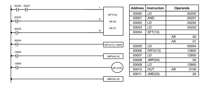
When a bit that is part of a shift register is used in OUT (or any other instruction that controls bit status), a syntax error will be generated during the program check, but the program will executed properly (i.e., as written).
