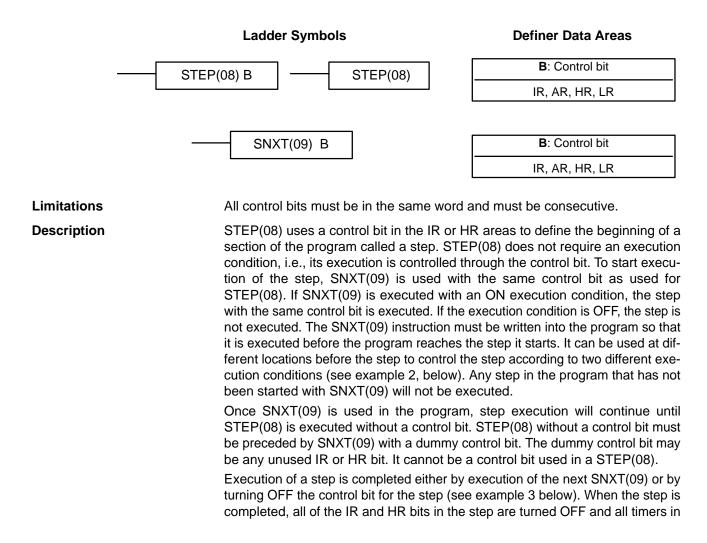
the step are reset to their SVs. Counters, shift registers, and bits used in KEEP(11) maintain status. Two simple steps are shown below.
