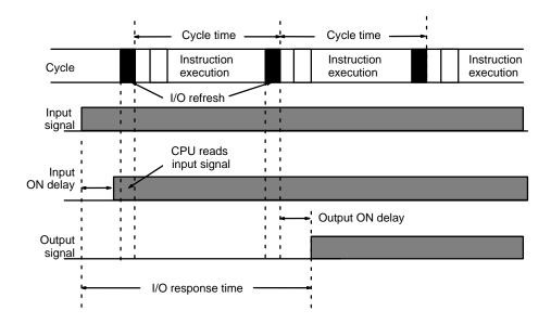
Minimum I/O response time = input ON delay + cycle time + I/O refresh time + output ON delay
