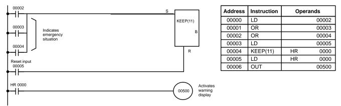
KEEP(11) can also be combined with TIM to produce delays in turning bits ON and OFF. Refer to *5-13-1 TIMER – TIM* for details.
