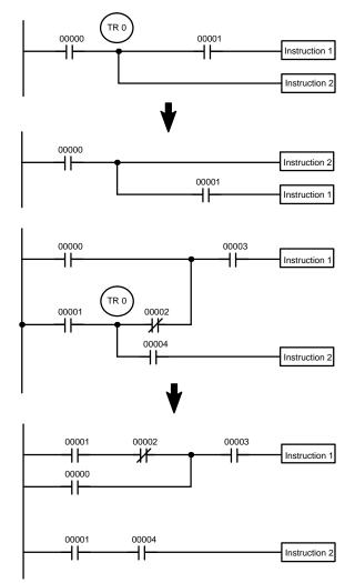
**Note** TR bits are only used when programming using mnemonic code. They are not necessary when inputting ladder diagrams directly, as is possible from a GPC. The above limitations on the number of branching points requiring TR bits, and considerations on methods to reduce the number of programming instructions, still hold.
