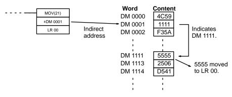
When using indirect addressing, the address of the desired word must be in BCD and it must specify a word within the DM area. In the above example, the content of \*DM 0000 would have to be in BCD between 0000 and 1999.
