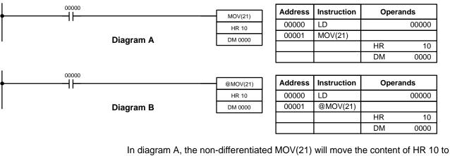
In diagram A, the non-differentiated MOV(21) will move the content of HR 10 to DM 0000 whenever it is cycled with 00000. If the cycle time is 80 ms and 00000 remains ON for 2.0 seconds, this move operation will be performed 25 times and only the last value moved to DM 0000 will be preserved there.
