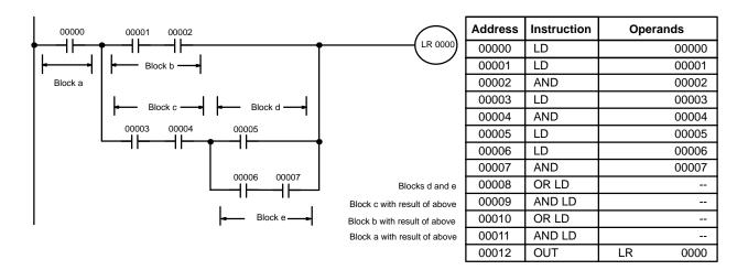
Again, this diagram can be redrawn as follows to simplify program structure and coding and to save memory space.
