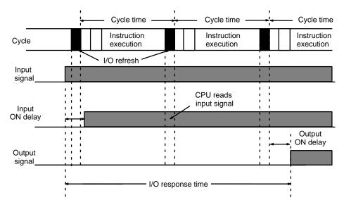
Maximum I/O response time = input ON delay + (cycle time x 2) + output ON delay
