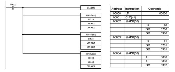
In the case below, 4F52A6E2 + EC3B80C5 = 13B8E27A7. The sum of the lower 4-digit addition is a 5-digit number, so CY (SR 25504) = 1, and the sum of the higher 4-digit addition is incremented by 1.
