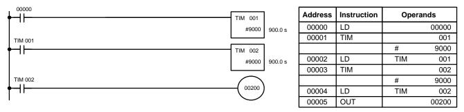
In this example, 00200 will be turned ON 30 minutes after 00000 goes ON. TIM can also be combined with CNT or CNT can be used to count SR area clock pulse bits to produce longer timers. An example is provided in *5-13-3 COUNTER* – *CNT*.
