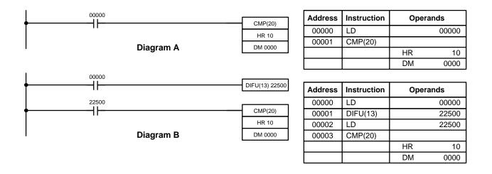
Example 2: Simplifying Programming Although a differentiated form of MOV(21) is available, the following diagram would be very complicated to draw using it because only one of the conditions
