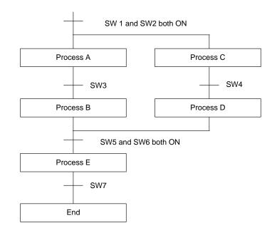
The program for this operation, shown below, starts with two SNXT(09) instructions that start processes A and C. These instructions branch from the same instruction line and are always executed together, starting steps for both A and C. When the steps for both A and C have finished, the steps for process B and D begin immediately.
